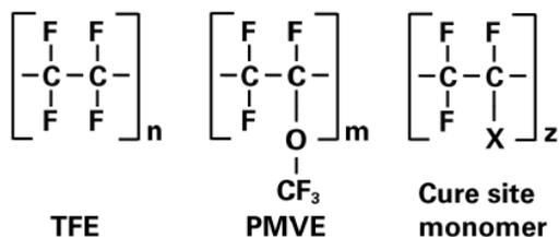
evolast® perfluoroelastomer compounds are based on terpolymers of tetrafluoroethylene (TFE), perfluoromethylvinyl ether (PMVE), and a cure site monomer (CSM). Thanks to the fully fluorinated monomers contained in perfluoroelastomers, they show superior chemical resistance.
